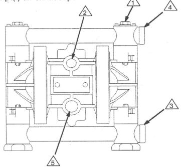
Note: the pump is supplied with fluid inlet and outlet ports facing the same direction. If required, the direction of one or both fluid ports may be changed. See Owners Manual 308 553.
